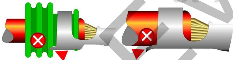
When processing single-wire seals, the cut-off tab (12) must not exceed a maximum length of 0.3 mm and must not damage the seals.
