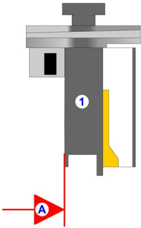
The surface (A) on the ram (1) is the reference surface for all assemblies in the crimping tool.
