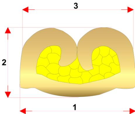
The crimp height (2) is an adjustable dimension in the processing tool. The crimp height is specified by the contact manufacturer depending on the conductor/cross section. As a non-destructive test, crimp height measurement offers reliable quality control during ongoing production.
