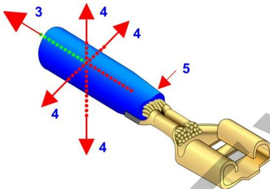
The pulling direction (3) must be made along the longitudinal axis of the contact and conductor! If the conductor would bend in one direction (4) directly after the wire crimping area, this would inevitably have an effect on the measuring result!
