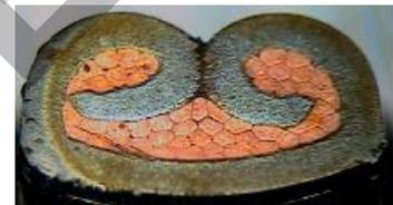
The crimp flanks are rolled in too far! Wrong assignment of crimp contact to conductor cross-section. The crimp contact is too large!
