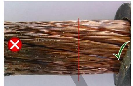
The color changes from a shiny orange-reddish shade to a matt dark brown surface, depending on the degree of oxidation (also called: passivating effect). This surface serves as a protective layer and prevents the penetration of oxygen or oxygen compounds such as water, thus stopping further corrosion and making copper very resistant to weathering.
