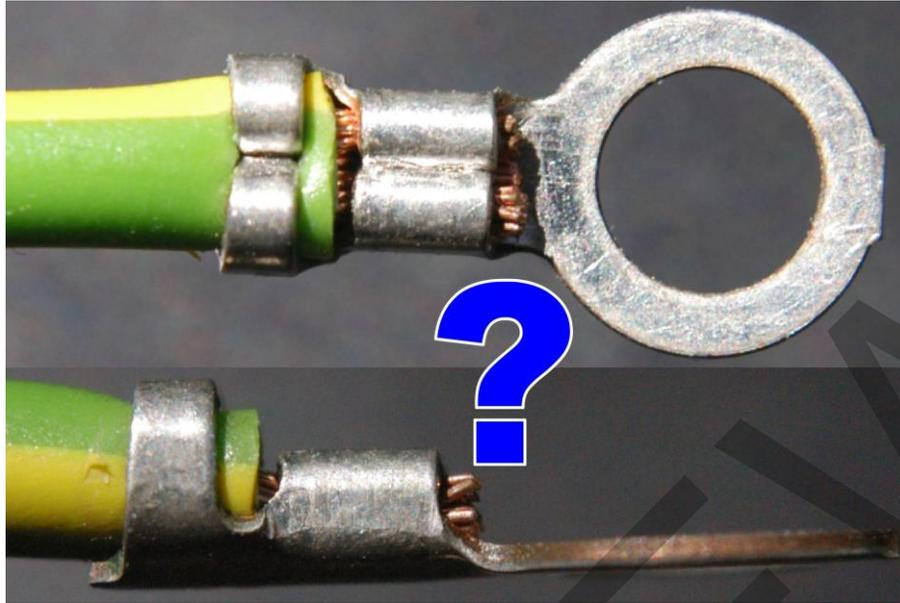
The assessment of the results of the individual work steps required for an ideal crimp connection is the bread and butter of wire processing. What is good, what is tolerable and what is bad? What consequences can faulty crimp connection have for the function of the wire harness? How can these faults be detected or avoided to begin with?
