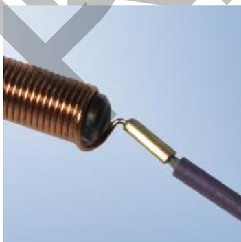
The design of the splice machine offers a operating range (A) in which very short connections can be processed. This is the great advantage of the splice technology with which electrical components can be connected with stranded conductors.
