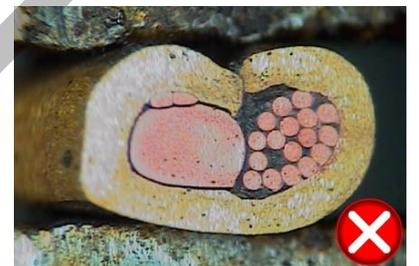
Of course, it is important that a created crimp also maintains its form. It's generally not a problem with the closed crimp barrel. But for the open crimp barrel the crimp form is key. When sheet metal is deformed, the material tends to spring back into its original shape after the bending process. This effect also occurs after the crimp flanks have been rolled in. To counteract this, the crimp flanks must touch and support each other (picture below: position A).
