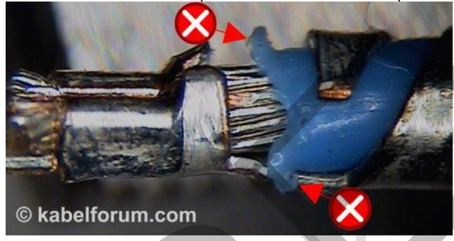
**Error:** Uncleanly cut, frayed insulation
