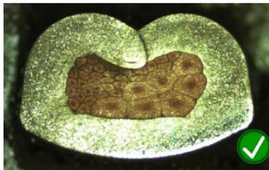
In crimping connection technology, this oxidized surface is undesirable because it has an electrically insulating effect and is responsible for increased transition resistances in a crimp connection. Due to the irregular pressing of the stranded conductor during the crimping process, this oxide layer is broken up. Together with the crimp contact, a friction-locked and keyed permanent connection with good electrical properties is created.
