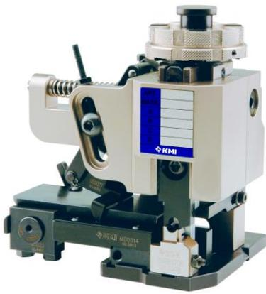
The ram (1) is guided in the base body (2) of the crimping tool. It must move easily and without play.
