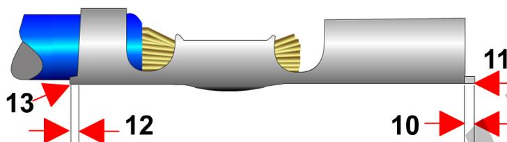
The cut-off tabs must be recognizable (at least 0.1 mm) and may be no longer than the thickness of the contact material. The length must not exceed 0.5 mm. The tabs must not be bent or deformed.
