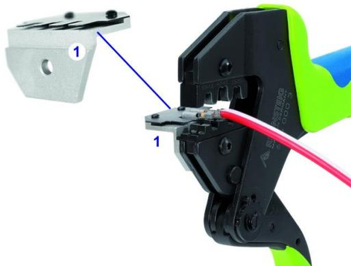
A correctly mounted positioning aid matched to the crimp contact is absolutely essential for creating a good crimp connection with hand crimping pliers.
