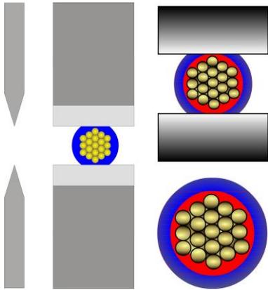
When stripping with standard hand strippers, mainly straight stripping blades are used.
