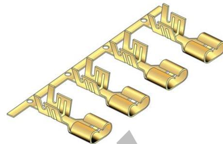
Neither the insulation crimp flanks nor the functional area of a crimp contact may be deformed or damaged! A visible cut-off tab means that the insulation crimp flanks or the functional area of the crimp contact did not come into contact with the cutter during the separation process. Consequently, damage or deformation of both areas can be excluded.
